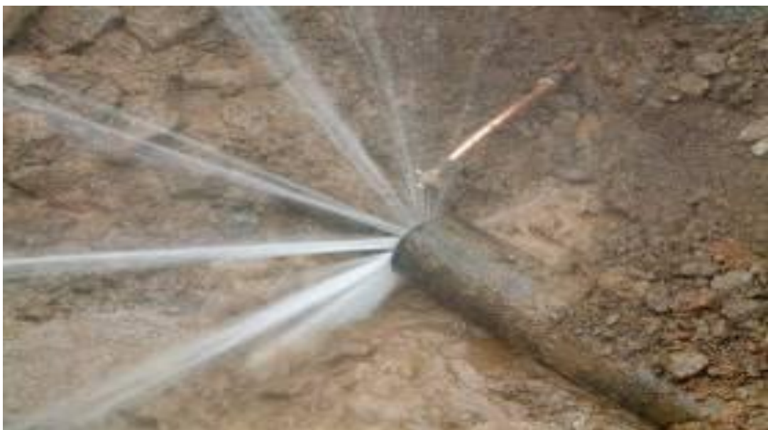
Figure 4.2: Water Leakage due to High Water Pressure
