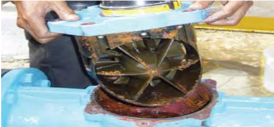
Figure 4.14 Sedimentation is a Major Source of Meter Recording Inaccuracy:
