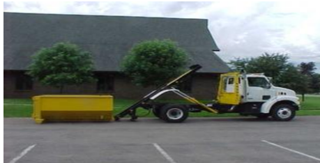
Figure 3: Hauled Container System (Source: EPA)
