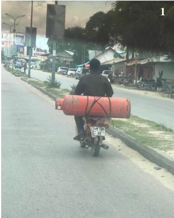
Picture 1: Show the LPG supplier transporting filled cylinder by using motorbike in horizontal position without covering the cylinder valves and he ignore to use PPEs.
