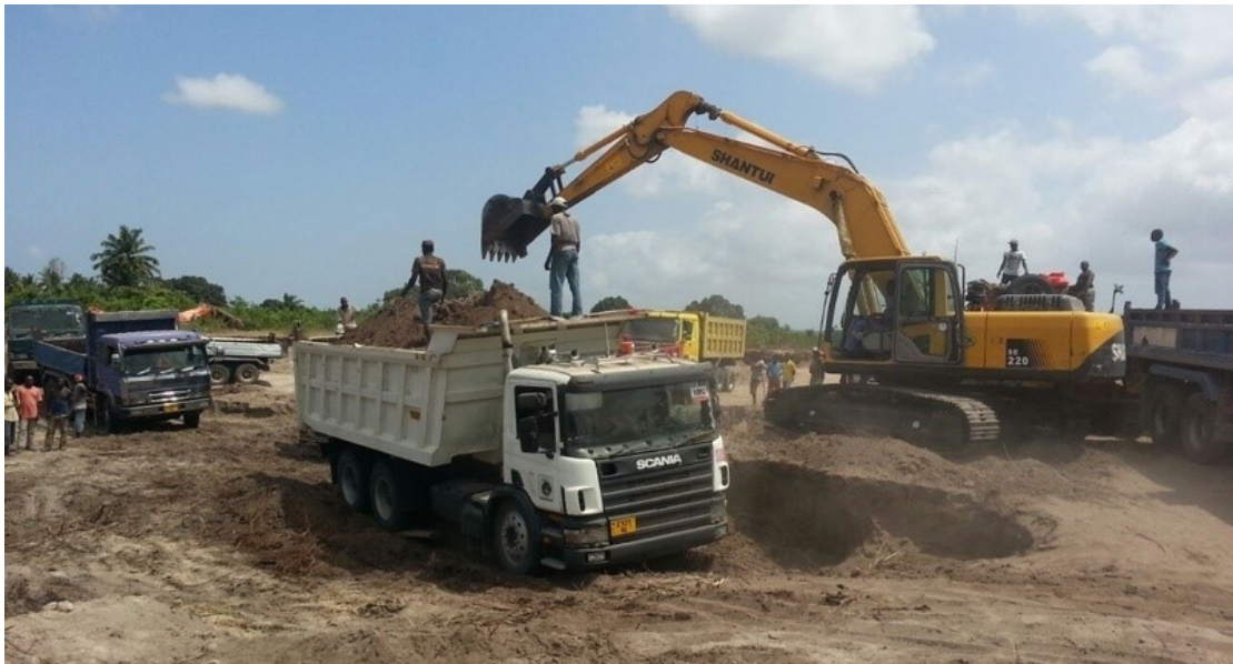
Figure 4.9: Sand Miners at Site ‘F’ Loading the Trucks with Sand using Excavator Machine
