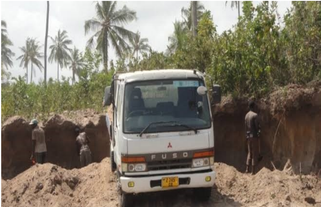
Figure 4.10: The Truck and the Sand Loaders Extracting Sand Manually at Site ‘C’.
