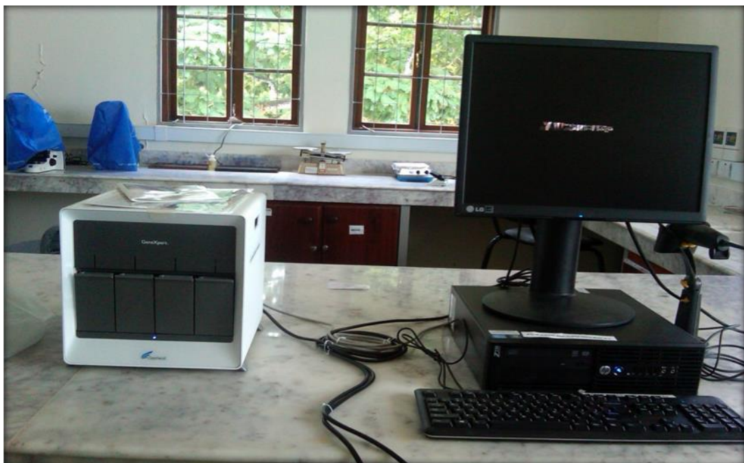
Figure 3.3: Gene Xpert MTB/RIF Machine
