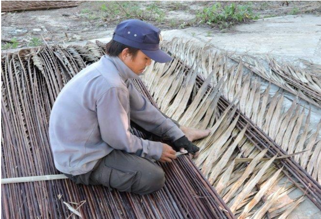
Figure 3.2: A Worker Is Seen Using Bamboo Strips To Fixate and Rim Coconut Leaves Into A Sheet of Coconut Thatch
